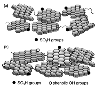
Figure 7. Structure of (a) PVC-activated carbon and (b) cellulose-derived activated carbon. Adapted from ref 65.
